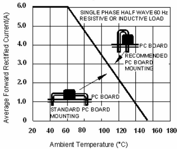
Fig. 2 — Maximum Forward Current Derating Curve
